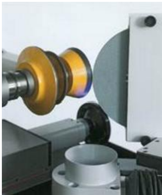
FIG. 3 Dressed Wheels and Dressing Wheel
