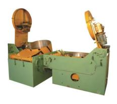
主要用于树脂结合剂固结磨具成型料混制。采用双锅结构设计,可以快速、均匀的完成混料。 Mainly used in the mixing of resin bond abrasive materials. The double pot structure can be used to complete the mixing quickly and evenly.
