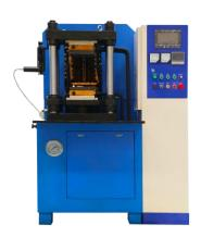
主要用于金属结合剂金刚石制品刀头、锯片等的热压烧结成型。液压系统采用伺服电机控制,压力控制精度高。控制系统采用 PLC、触摸屏,操作简单、方便。Mainly used for hot-pressing sintering forming of metal bond diamond product bit, saw blade, etc. The hydraulic system is controlled by a servo motor with high pressure control accuracy. The control system adopts PLC, touch screen, simple and convenient operation.
